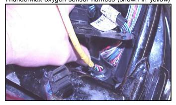
connector through the opening between the frame and the caddy, exiting behind the right wing of the oil tank.
