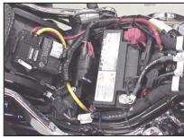
attach the fuse box to the plastic fuse box bracket.
