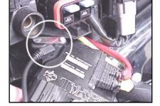
out far enough for temporary attachment of the ECM communication cable for map programming adjustments.
