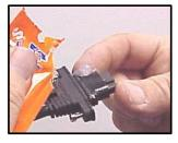
FX/FLST-I: Install the ThunderMax ECM onto the ECM caddy; insert the oxygen harness connector into the ECM with the imprinted "ThunderMax" logo facing up. Tighten the (2) Phillips connector screws. Lift ECM and install the two 18-pin connectors, ensuring they are fully seated and latched. Replace ECM into the caddy.
